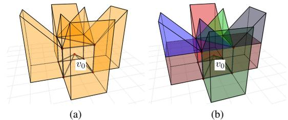
Fig. 5. (a)  $\mathcal{C}_{free}^{v_0}(q^{v_0})$  is bounded by polygons. (b)  $\mathcal{C}_{free}^{v_0}(q^{v_0})$  is decomposed into multiple convex polyhedrons.
