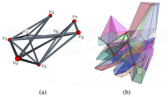
Fig. 8. (a) A VTT is constructed from 17 members with 8 nodes. (b)  $C_{free}^{v_7}(q_i^{v_7})$  is decomposed into 56 cells in total.
