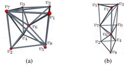
Fig. 10. The motion task is to change the shape of a VTT from (a) a cubic truss for rolling locomotion to (b) a tower truss for shoring.
