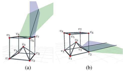
Fig. 4. (a) The intersection between the polygon generated by node  $v_1$  with member  $(v_6, v_8)$  and the polygon by node  $v_2$  with member  $(v_6, v_7)$  is a ray. (b) The intersection between the polygon generated by node  $v_1$  with member  $(v_2, v_3)$  and the polygon by node  $v_4$  with member  $(v_2, v_3)$  is also a polygon which is the region between the two parallel black lines.
