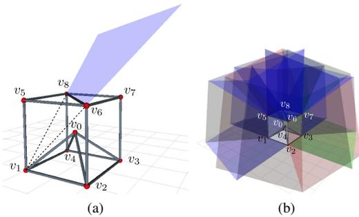
Fig. 2. (a) Given node  $v_0$ , one of its neighbors  $v_1$  and a member  $(v_6, v_8)$  can define the blue polygon. This polygon is part of  $C_{obs}^{v_0}$ . (b) The obstacle region  $C_{obs}^{v_0}$  of  $v_0$ .
