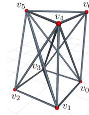
Fig. 7. A VTT Constructed by 18 Members
