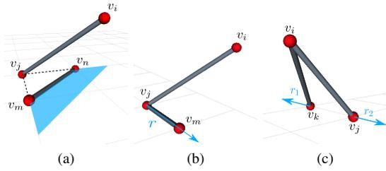
Fig. 1. (a)  $(v_i, v_j)$  collides with  $(v_m, v_n)$  when  $v_i$  is on the blue polygon. (b)  $(v_i, v_j)$  collides with  $(v_m, v_j)$  when  $v_i$  is on the blue ray  $r$ . (c)  $(v_i, v_j)$  collides with  $(v_i, v_k)$  when  $v_i$  is on the blue ray  $r_1$  or  $r_2$ .
