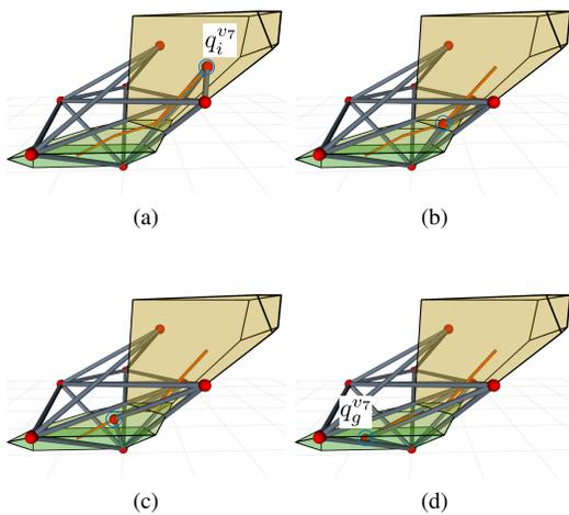
Fig. 9. The task is to move node  $v_7$  from its initial configuration  $q_i^{v_7}$  shown in (a) to a goal configuration  $q_g^{v_7}$  shown in (d). The three cells and the complete path node  $v_7$  has to traverse are shown.  $v_7$  is moved to the intersection between the first cell and the second cell shown in (b), then to the center of the second cell shown in (c), and finally to the goal location inside the third cell.
