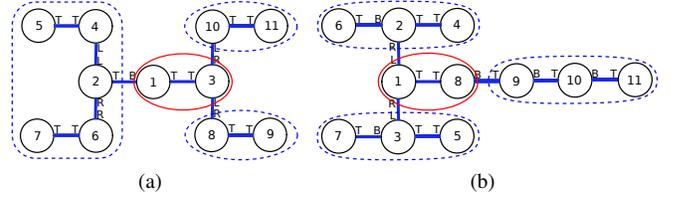
Fig. 10. (a) Graph representation of walker configuration and (b) graph representation of mobile manipulator configuration.  $MCS(1, 1)$  is encircled by “—” under mapping  $1 \rightarrow 1$  and  $3 \rightarrow 8$ . After removing  $MCS(1, 1)$ , there are three unconnected subgraphs in both the current initial configuration and goal configuration which are encircled by “- -”.
