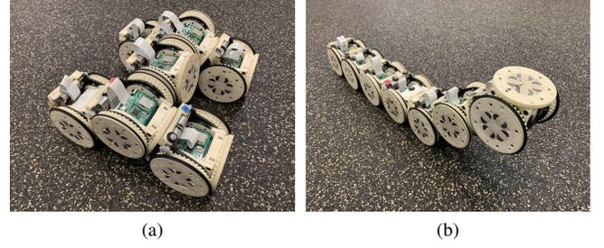
Fig. 15. Reconfigure a driver configuration (a) into a snake configuration (b) with seven SMORES-EP modules involved.
