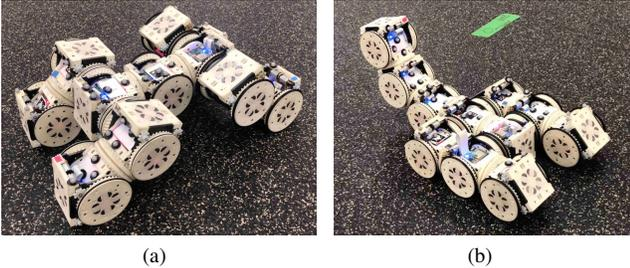
Fig. 9. Reconfigure a walker configuration (a) into a mobile vehicle with an arm configuration (b) with eleven SMORES-EP modules involved.
