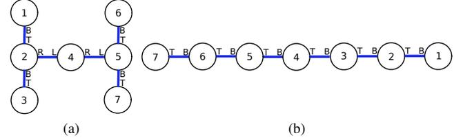
Fig. 16. (a) Graph Representation of Driver Configuration and (b) Graph Representation of Snake Configuration.
