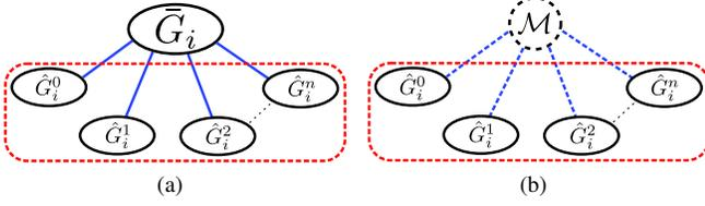
Fig. 7. Replace  $\bar{G}_i = (\bar{V}_i, \bar{E}_i)$  with virtual module  $\mathcal{M}$  and replace connections between  $\bar{G}_i = (\bar{V}_i, \bar{E}_i)$  and every  $\hat{G}_i^\alpha = (\hat{V}_i^\alpha, \hat{E}_i^\alpha)$  with virtual connections.
