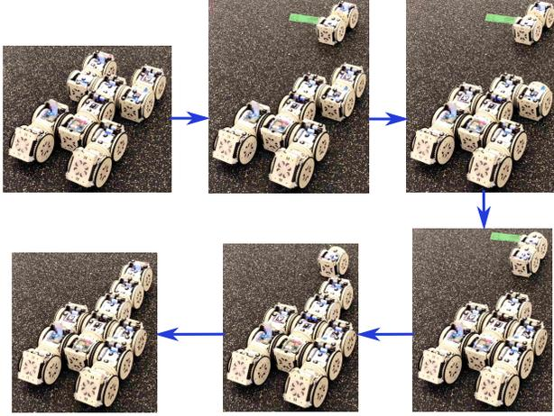
Fig. 14. SMORES-EP hardware reconfiguration from a walker to a mobile vehicle with an arm.
