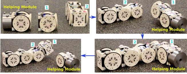
Fig. 8. A helping module docks with Module 1 BOTTOM Face and lifts it up so that LEFT Face of Module 1 can be aligned with BOTTOM Face of Module 2, then carry Module 1 to the location to finish the docking action.
