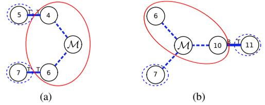
Fig. 12.  $MCS(\mathcal{M}, \mathcal{M})$  is encircled by “—” under mapping  $\mathcal{M} \rightarrow \mathcal{M}$ ,  $4 \rightarrow 6$  and  $6 \rightarrow 10$ . After removing  $MCS(\mathcal{M}, \mathcal{M})$ , there are two unconnected subgraphs in both the current initial configuration and current goal configuration which are encircled by “- -”.
