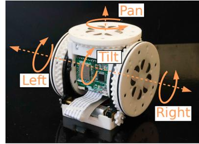
Fig. 1. A SMORES-EP module with four active rotational degrees of freedom and four connectors using an array of electro-permanent (EP) magnets.
