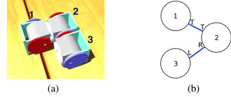
Fig. 4. (a) Three-Module Configuration and (b) Three-Module Configuration Graph.
