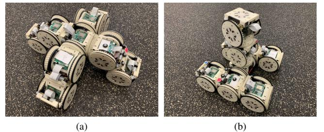
Fig. 17. Reconfigure a omni-driver configuration (a) into a mobile observer configuration (b) with nine SMORES-EP modules involved.
