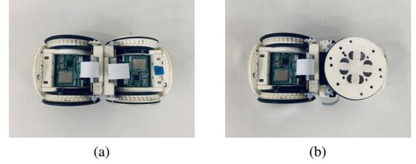
Fig. 3. Connection between two BOTTOM Faces: (a) Orientation is 0 and (b) Orientation is 1.
