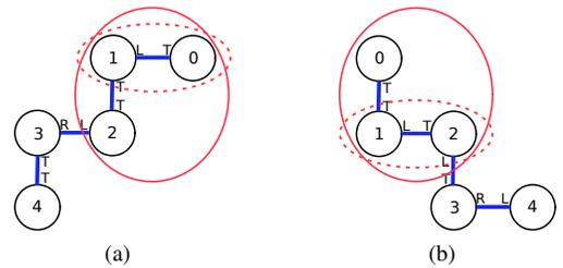
Fig. 5. Two SMORES-EP configurations are shown. The subgraphs of (a) and (b) circled by “- -” is an example of common subconfiguration with mapping  $1 \rightarrow 1$  and  $0 \rightarrow 2$ . The subgraphs of (a) and (b) circled by “—” is  $\text{MCS}(1, 1)$  with mapping  $1 \rightarrow 1$ ,  $2 \rightarrow 0$  and  $0 \rightarrow 2$ .
