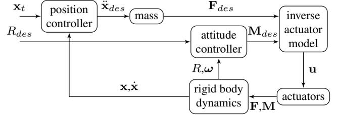
Fig. 7. Fully actuated trajectory and orientation control.
