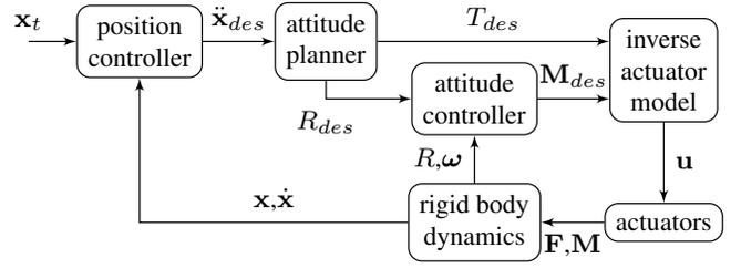
Fig. 6. Conventional trajectory control for underactuated quadrotor.
