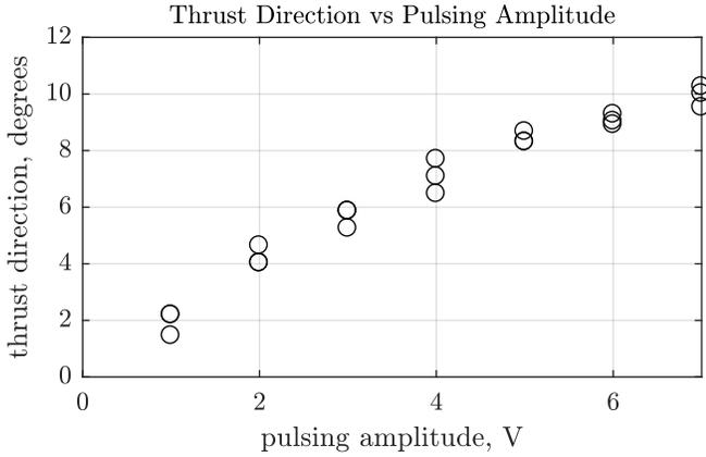
Fig. 5. Bench measurements of lateral forces and increasing voltage modulation amplitude.
