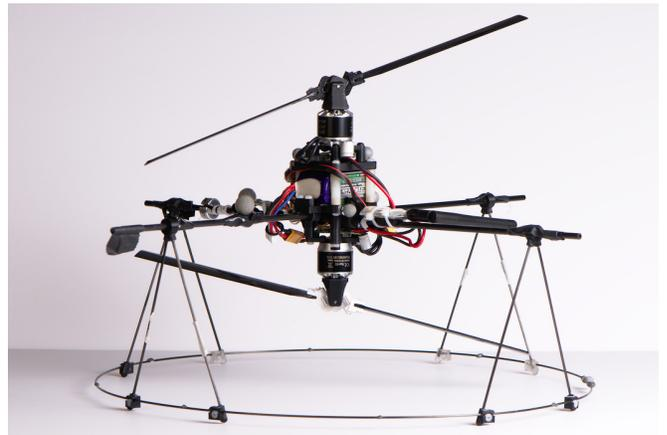
Fig. 4. Coaxial helicopter.
