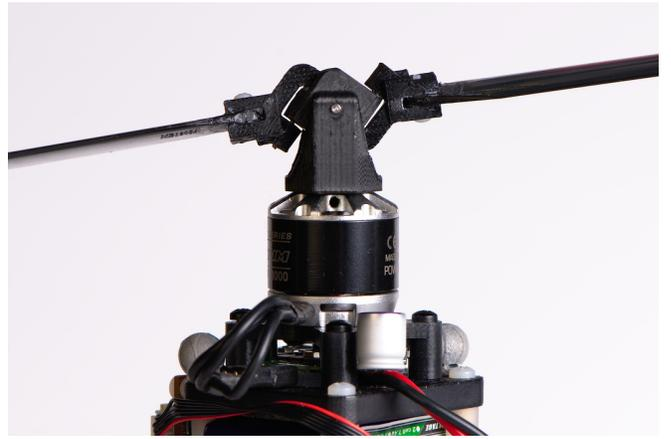
Fig. 3. Top rotor of coaxial helicopter.
