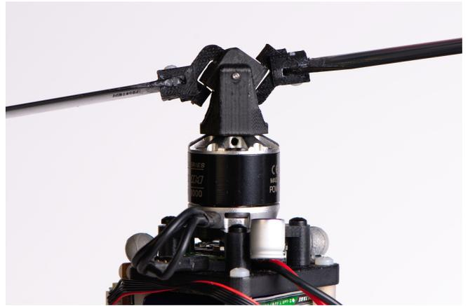
Fig. 3. Top rotor of coaxial helicopter.
