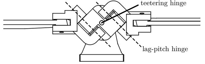
Fig. 2. Teetering rotor with skewed lag-pitch hinges.
