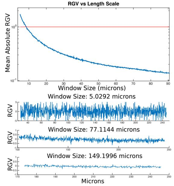
Fig. 6. Top: Plot of mean absolute RGV with increasing window size. Red line indicates resolution limit,  $|\overline{RGV}|(w) = 1$ . Right: Bottom of RGV computed on the same dataset with different window sizes. We can see that the data becomes smoother with increasing window size.
