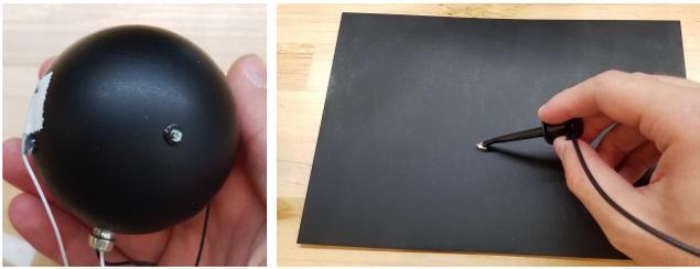
Fig. 9. Left: Spherical PaintPot that senses position on the top hemisphere. Right: Flat-sheet PaintPot capable of sensing the X-Y position of the wiper.
