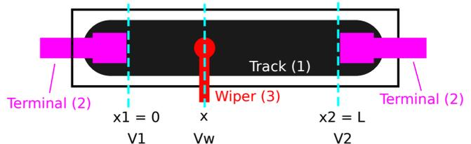
Fig. 1. Potentiometer schematic showing the three parts (track, terminals, and wiper) as well as position and voltage labels.
