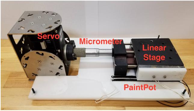
Fig. 7. Testing setup used to evaluate RGV and hysteresis.
