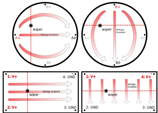
Fig. 10. Top: Top-down view of voltage gradients on the sphere PaintPot. Bottom: Voltage gradients on sheet PaintPot.
