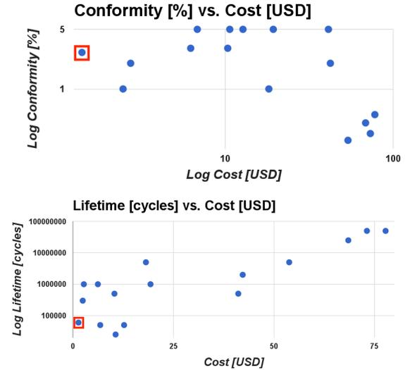
Fig. 8. Plots of cost vs. conformity and cost vs. lifetime for commercial potentiometers with features similar to the wheel PaintPot ( $360^\circ$  sensing range and continuous rotation). PaintPot marked with red square.
