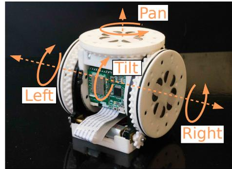
Fig. 3. SMORES-EP module with labeled joints. The module is the size of an 80mm cube.
