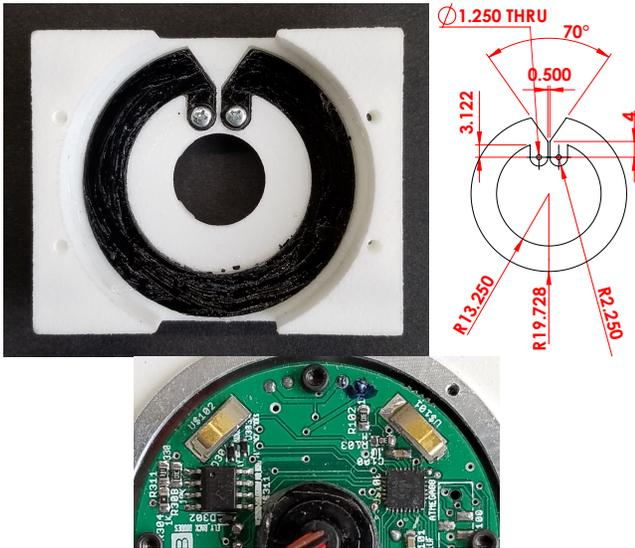
Fig. 4. Top Left: Wheel PaintPot installed in chassis. Top Right: Drawing of wheel PaintPot with dimensions in mm. Bottom: Circuit board used with wheel PaintPots showing Harwin S1791-42 wipers mounted at a  $50^\circ$  angle.
