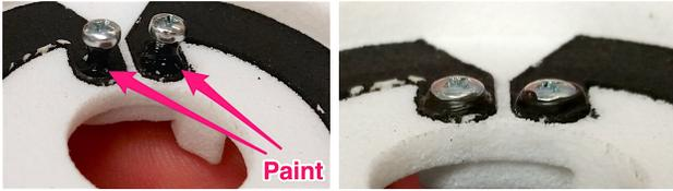
Fig. 2. A bead of conductive paint applied beneath the screw head forms a good electrical connection with the track.
