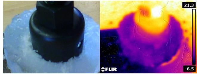
Fig. 3. Left: A hole saw cutting a hole in the ice blank. Right: A heat map (in °C) of the drill and ice blank.
