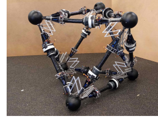
Fig. 1. The hardware prototype of a VTT in cubic configuration is composed of 12 members. Note that at least 18 members are required for topology reconfiguration [18].
