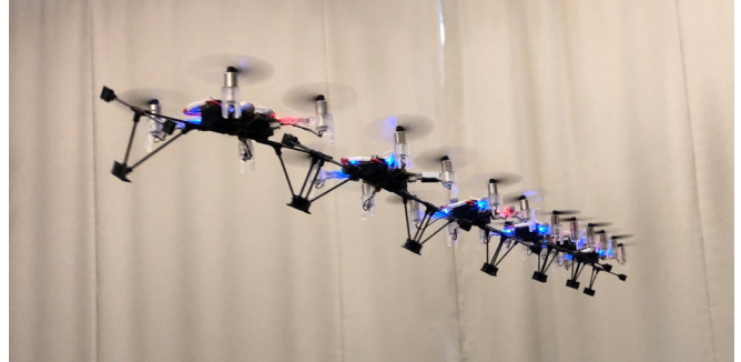
Fig. 1. Six modules flying in a line configuration.
