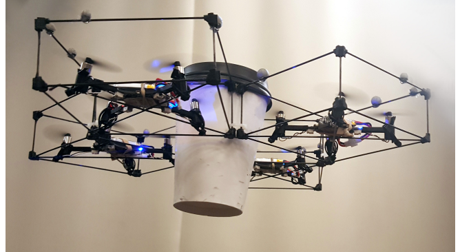
Fig. 1. The Flying Gripper holding a coffee cup in midair.
